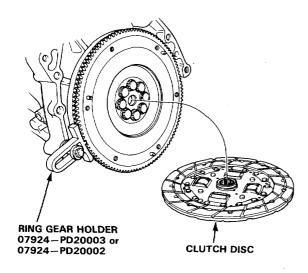
3. Measure the clutch disc thickness.
